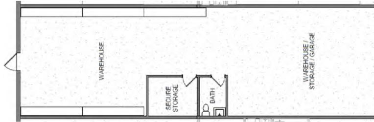
The standard open plan provides maximum access with two roll up doors and a wide open shell. Unit comes complete with air conditioned bath and secure storage room.
